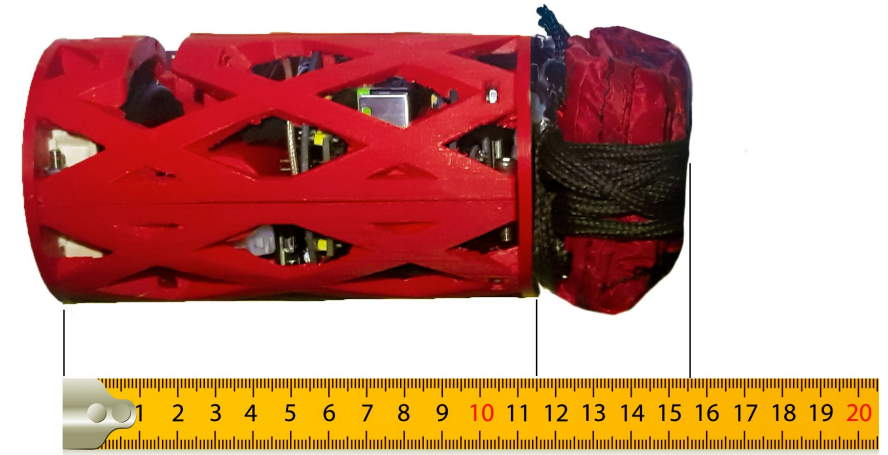
Effective dimensions of the CanSat
