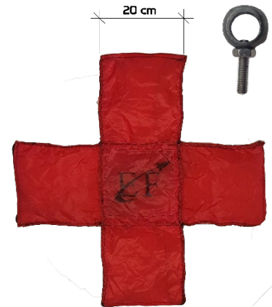
Fig. 10 Parachute top view and eyebolt attachments
