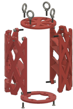
Fig. 3 Case exploded view
