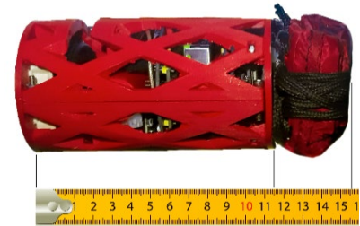
Fig. 11 Folded parachute size
